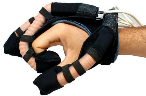
Figure 1.2 - (a) ExoHand Festo. [6] (b) Soft Robotic Glove Wyss Institute [7].
